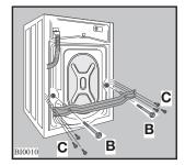
5. Remove the bracket **D** and refit the six smaller bolts C.
